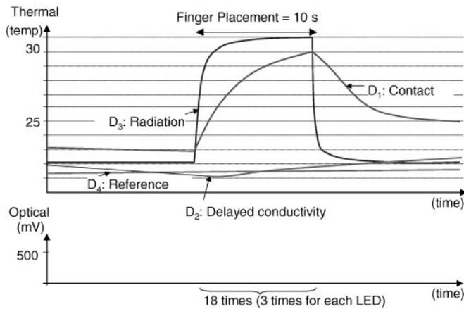
Fig. 5. Example of signals from the sensor pickup. Thermal and optical signals are continuously collected before/after finger placement.
