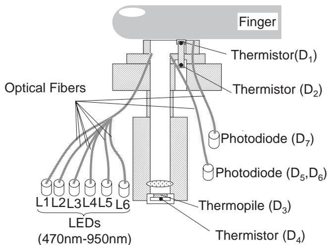
Fig. 4. Structure of sensor pickup.
