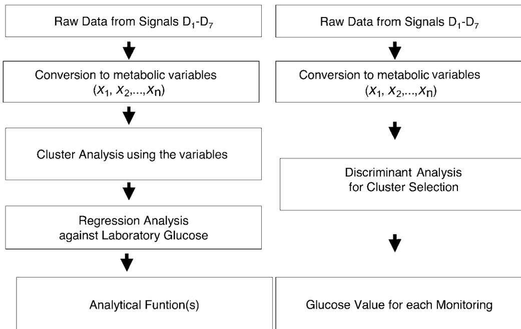
Fig. 6. Calibration process and estimation of glucose value. Flow diagram depicting the calibration process (left-hand side) and glucose calculation (right-hand side).
