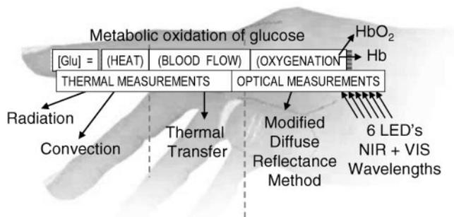
Fig. 1. Principles of the MHC method.
