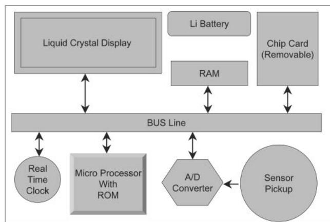
Fig. 2. Block diagram of the MHC device.
